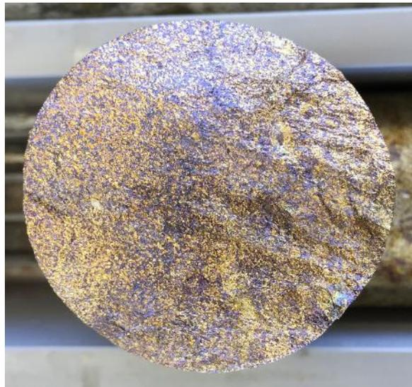
**Plate 1. Cross section through NQ2 core showing bornite disseminated in the matrix of the sulphides (359.3 metres down hole).**
