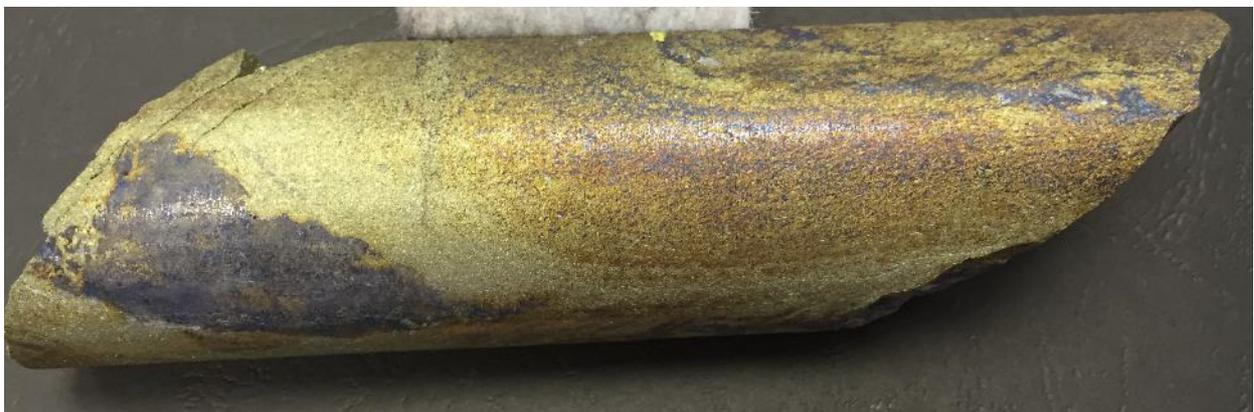
**Plate 2. NQ2 core showing bornite in foliation (right) and rimming pyrite and pyrrhotite (left) (351m down-hole).**
