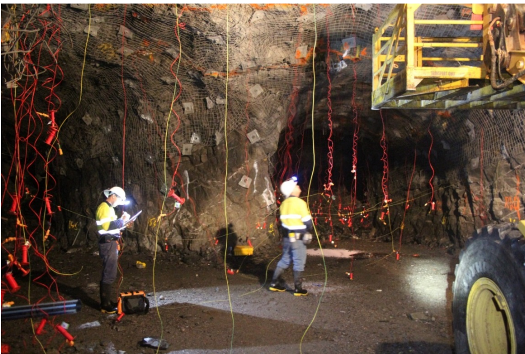
Figure 10 - Stope Charging Karari Underground 2190 Hangingwall lode
