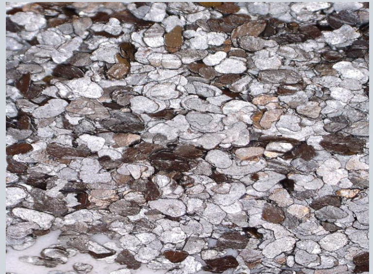
Jumbo graphite flakes obtained from Ancuabe rock chip samples
