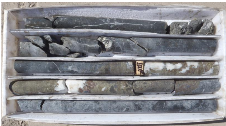
Figure 3: LV5DD007. Massive sulphide from 99.1m to 100.6m in fractured and altered Juarez Limestone unit (Tres Amigos).
