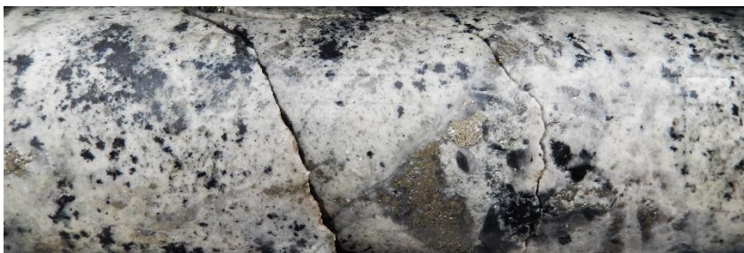
Figure 8: LEFT Core photo at 587m (CH-DDH027). The monzodiorite is highly altered (phyllic) with tourmaline rosettes and sulphide replacements. The sulphides occur as patches, veins and as disseminations.
