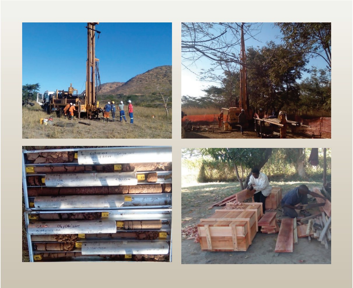
Figure 2: Showing hydrological drilling near the base of Panda Hill (top left), drilling for geotechnical samples in the TSF region (top right), geotechnical core samples (bottom left) and carpenters preparing boxes to transport the samples to South Africa (bottom right).
