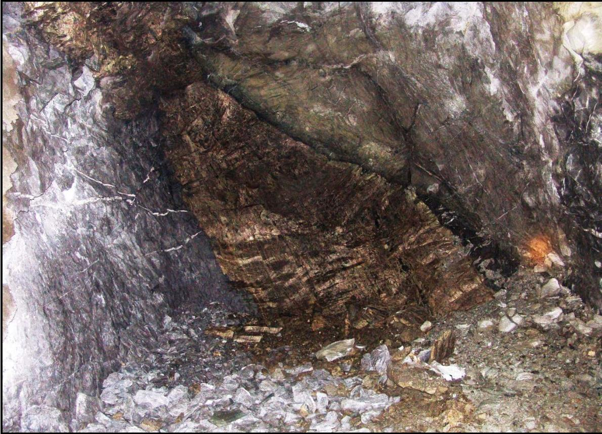
**Figure 3: Goose 10170 level (now mined) showing high grade massive nickel sulphide (~13% Ni) in the ore drive.**
