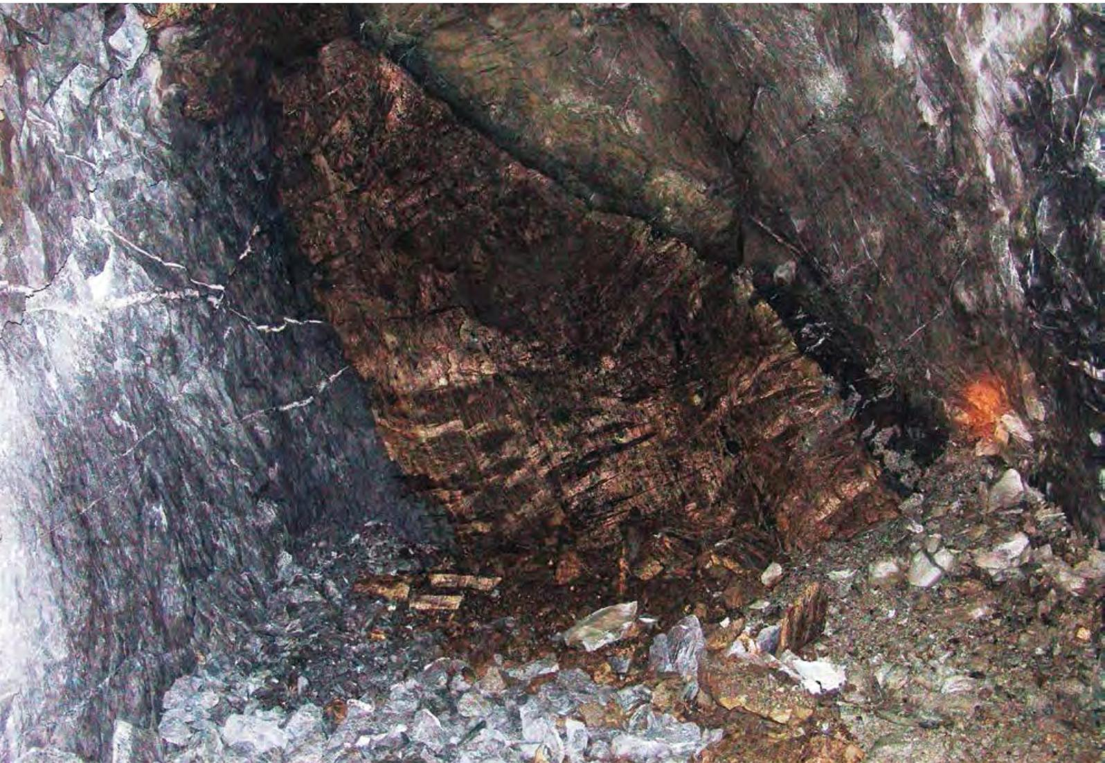
*Silver Swan: Goose 10170 level (now mined) showing high grade massive nickel sulphide (~13% Ni) in the ore drive.*
