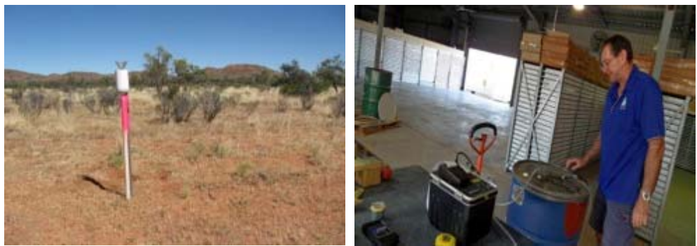
Image 3 (left): Air quality sampling station at the Nolans Site. Image 4 (right): Radioactive gas emission testwork on mineralised and waste rock samples being completed offsite.
