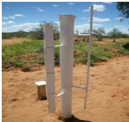
Image 5: Rising stage sampler installed at the Nolans Site for the collection of water samples from an ephemeral creek.
