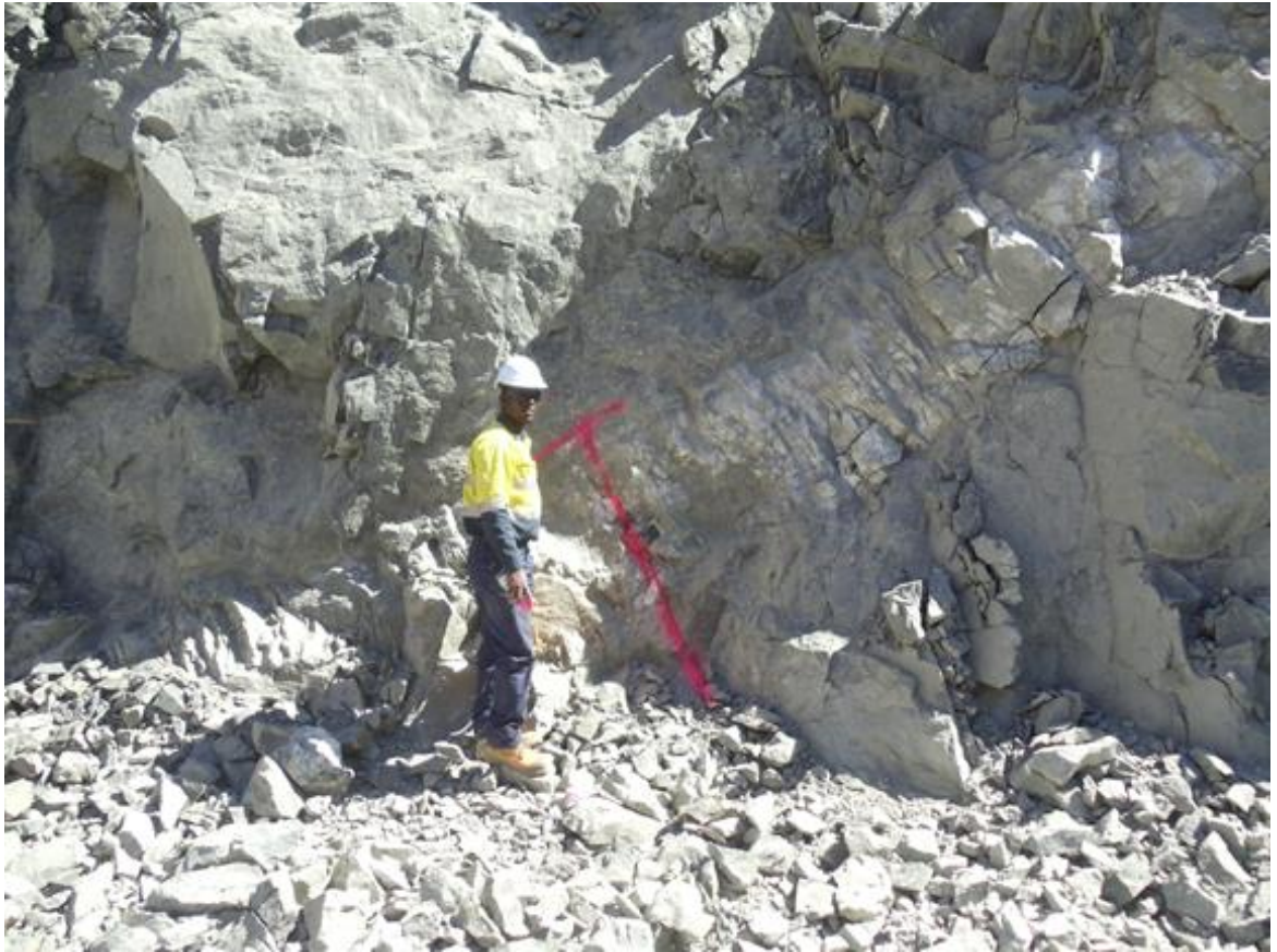
Figure 5 Photograph of Parrot Feathers Vein Exposed in Lindsays Pit, Showing Shallow Dip, 1m Width and Sample Point
