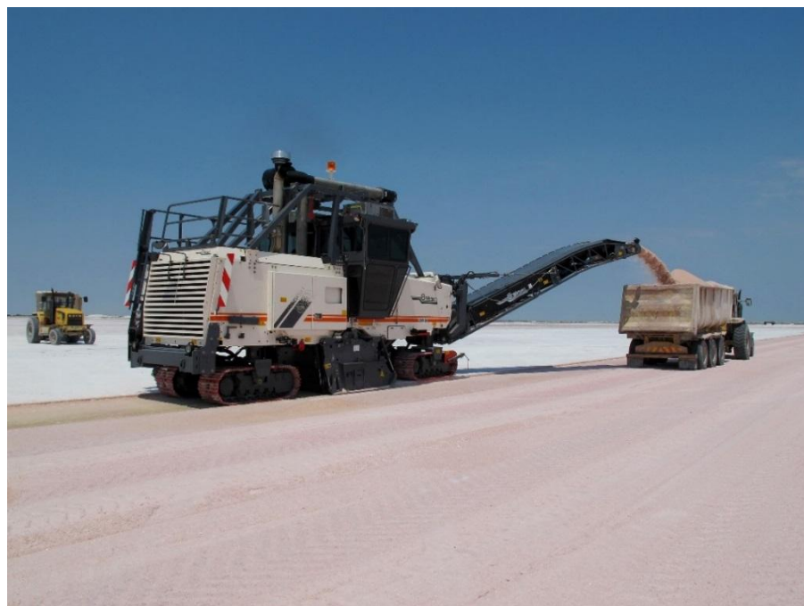
Figure 5 – The DFS is focussing on Wirtgen surface miners that are used extensively in salt mining – Shown here in Botash, Botswana. (Note: not a Danakali project)
