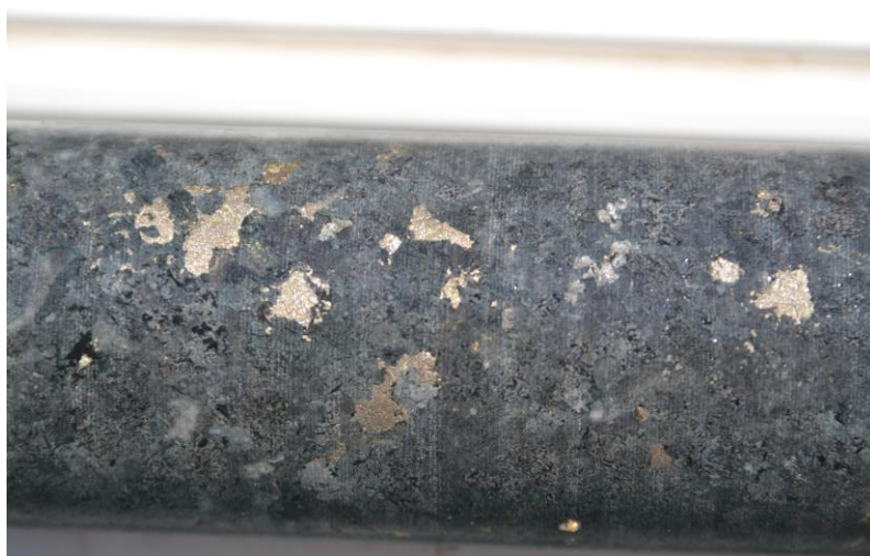
FIGURE 2: Globular sulphides within coarse grained mesocumulates at around 206 metres downhole in MRDD008.
