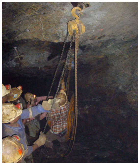
Block 30 raise: Reeling wheel of the new loader being lowered into Block 30
