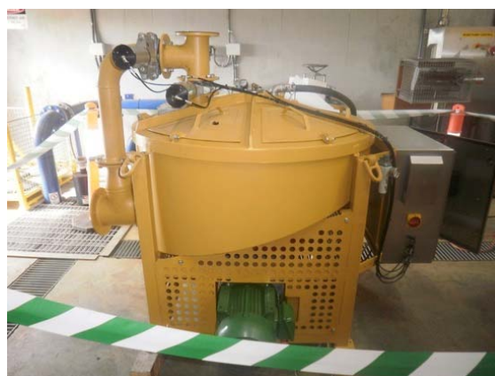
Figure 2 – Pressure Jig – high mass pull gravity gold recovery (left) and In-line Spinner – centrifugal gravity gold recovery (right) at Gekko Systems in Australia
