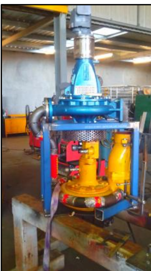
Photograph 2. Submersible dredge pump under construction in Perth, W.A., prior to shipping to site.
