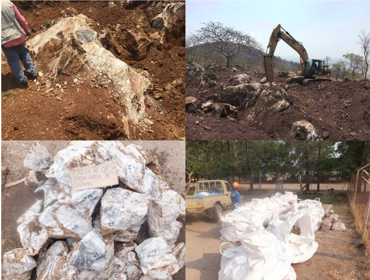
Figure 2: Showing fresh carbonatite outcrop from the initial starter pit area (top left), rock breaker at work (top right), bulk samples collected (bottom left) and 1 tonne bagged bulk sample ready for shipment (bottom right).
