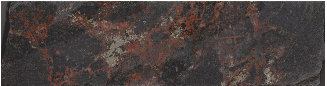
FC2 Prospect: Close-up of MMA010 drill core (cut) at 249.7m DH showing breccia texture, magnetite, actinolite, albite, pyrite, chlorite and red feldspar in matrix (and alteration), and apparent albite alteration of host.
