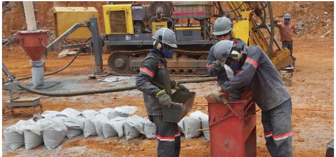
Cleaning splitter for sample preparation
