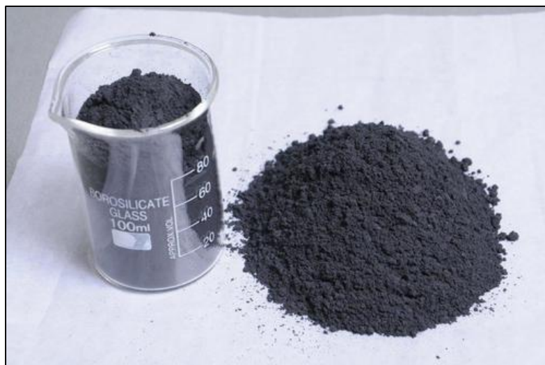
Figure 7. Example of reduced Graphene Oxide powder ( www.indiamart.com/united-nanotech/industrial-chemical.html )
