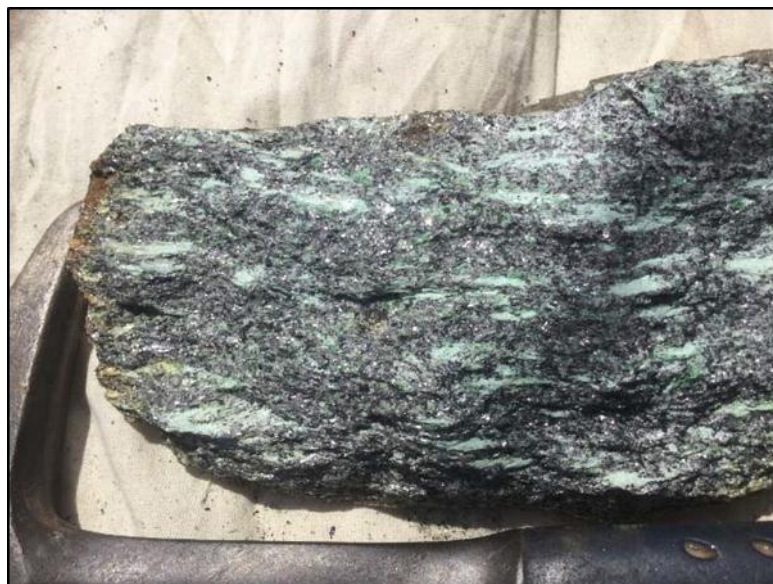
Plate 1. Pit BL002 (sample ID BS010) showing graphite-sericite-quartz schist which returned 9.29% TGC and 0.16% vanadium with coarse flake material.
