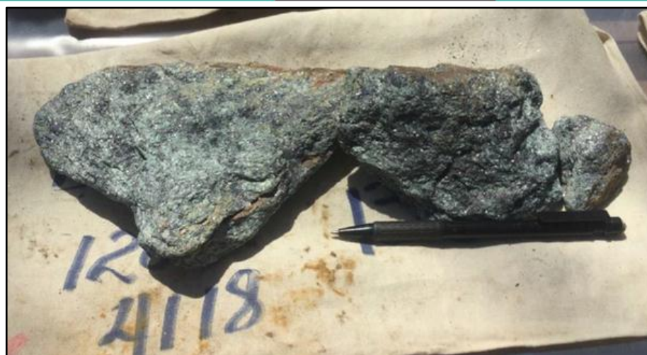
Plate 2. Pit 13C (sample ID BS012) taken 1.2m below surface with high grade graphite-sericite-schist which returned 9.91% TGC and 0.11% vanadium.
