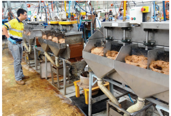
Figure 9: Beneficiation pilot plant barite prefloat circuit in operation.
