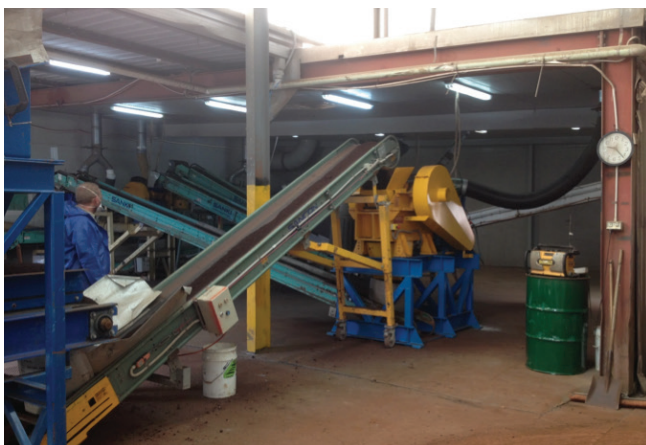
Figure 6: Crushing and screening of sample
