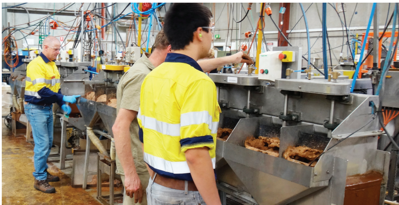
Figure 1: Commissioning of the barite prefloat circuit
