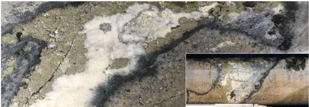
Figure 4: ABOVE Close-up core photo at 450.9m (CH-DDH027) Silicified phyllic-altered volcanics hosting quartz-carbonate veins with pyrite-chalcopyrite-arsenopyrite. The veins typically have a tourmaline rim. INSERT Core photo of the same interval pre core-cutting. BELOW Close-up core photo at 451.3m (CH-DDH027) A similar vein as at 450.9m with more distinct potassic alteration (pink colouration) surrounding the vein.
