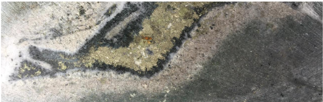
Figure 4: ABOVE Close-up core photo at 450.9m (CH-DDH027) Silicified phyllic-altered volcanics hosting quartz-carbonate veins with pyrite-chalcopyrite-arsenopyrite. The veins typically have a tourmaline rim. INSERT Core photo of the same interval pre core-cutting. BELOW Close-up core photo at 451.3m (CH-DDH027) A similar vein as at 450.9m with more distinct potassic alteration (pink colouration) surrounding the vein.
