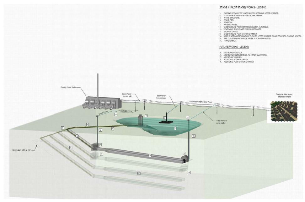
Attachment 2 - Concept Diagram for Final Stage of Solar-Pumped Hydro Project
