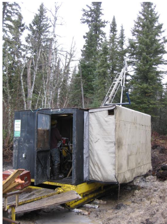
Figure 1: Drill rig commencing diamond drilling program at Manitowadge graphite project in Ontario, Canada
