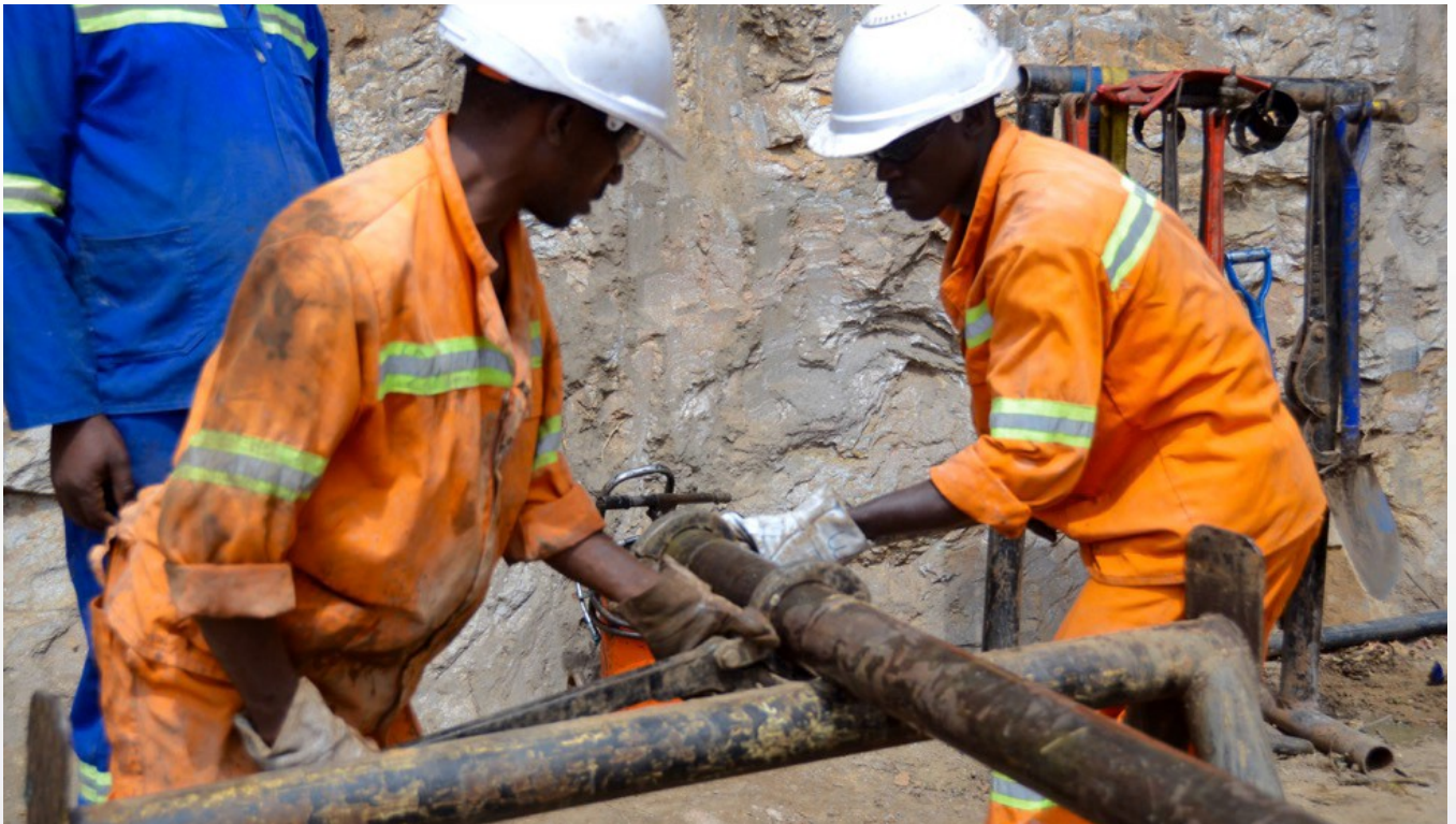
Photo 1. Diamond drilling underway at DD16, Ulanzi. Rock face behind drillers is graphitic outcrop.
