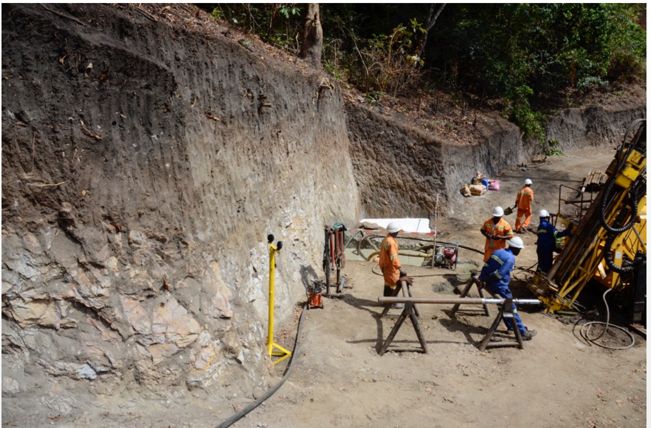
Photos 2 (above) and 3 (below) - Diamond drilling underway at DD16, Ulanzi, midway upslope of the Ulanzi ridge. Photos face north and show 1-2m of graphitic soil overlaying the graphite mineralised structure.
