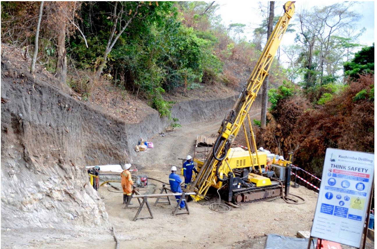
Photos 2 (above) and 3 (below) - Diamond drilling underway at DD16, Ulanzi, midway upslope of the Ulanzi ridge. Photos face north and show 1-2m of graphitic soil overlaying the graphite mineralised structure.
