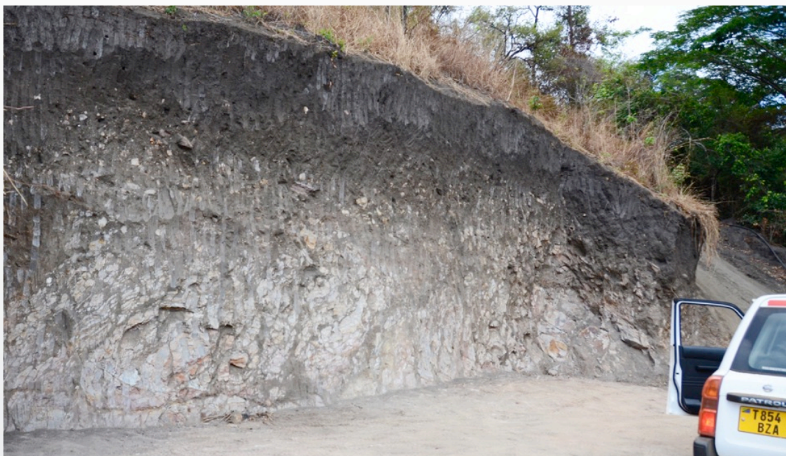
Photo 6. Ulanzi drill pad prepared for current programme showing 1.5m of graphitic soil over graphite mineralised structure.
