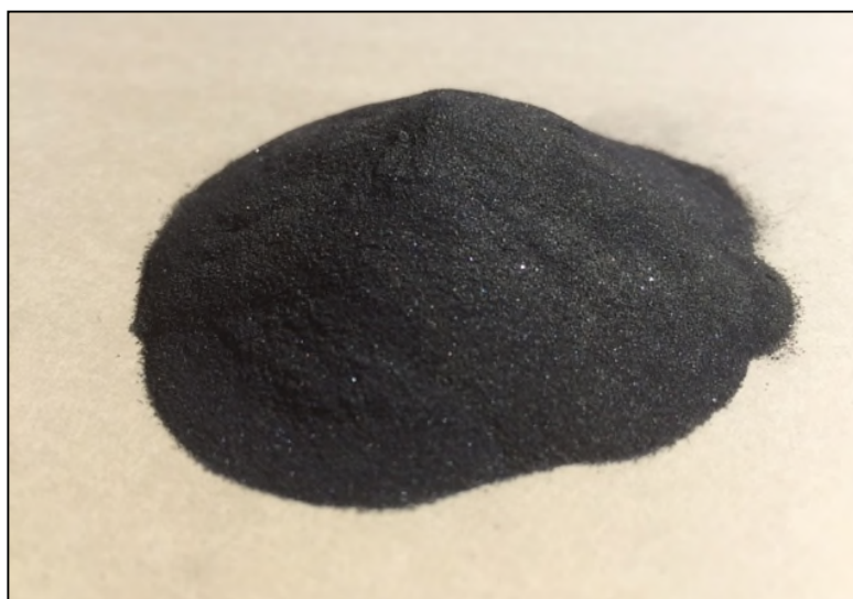
Figure 5: MAHUMO CONCENTRATE: 51.9% Cu & 1,300ppm Ag produced from test work on sulphide ores (Refer previous announcements: 6 July 2015, 31 July 2015)
