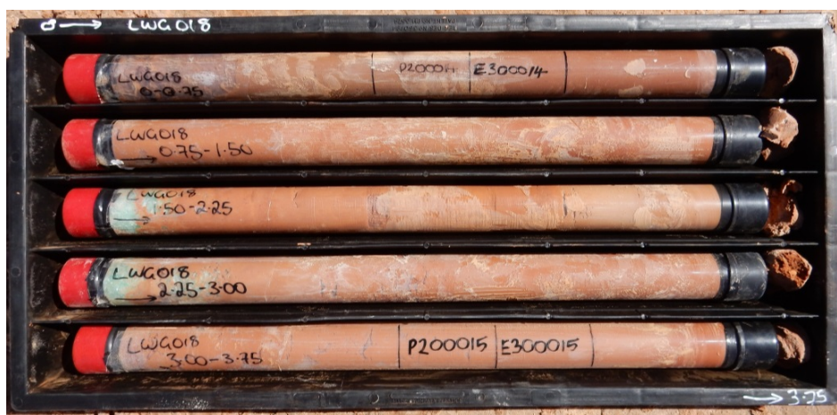
Figure 5: Intact Core Sample Tubes
