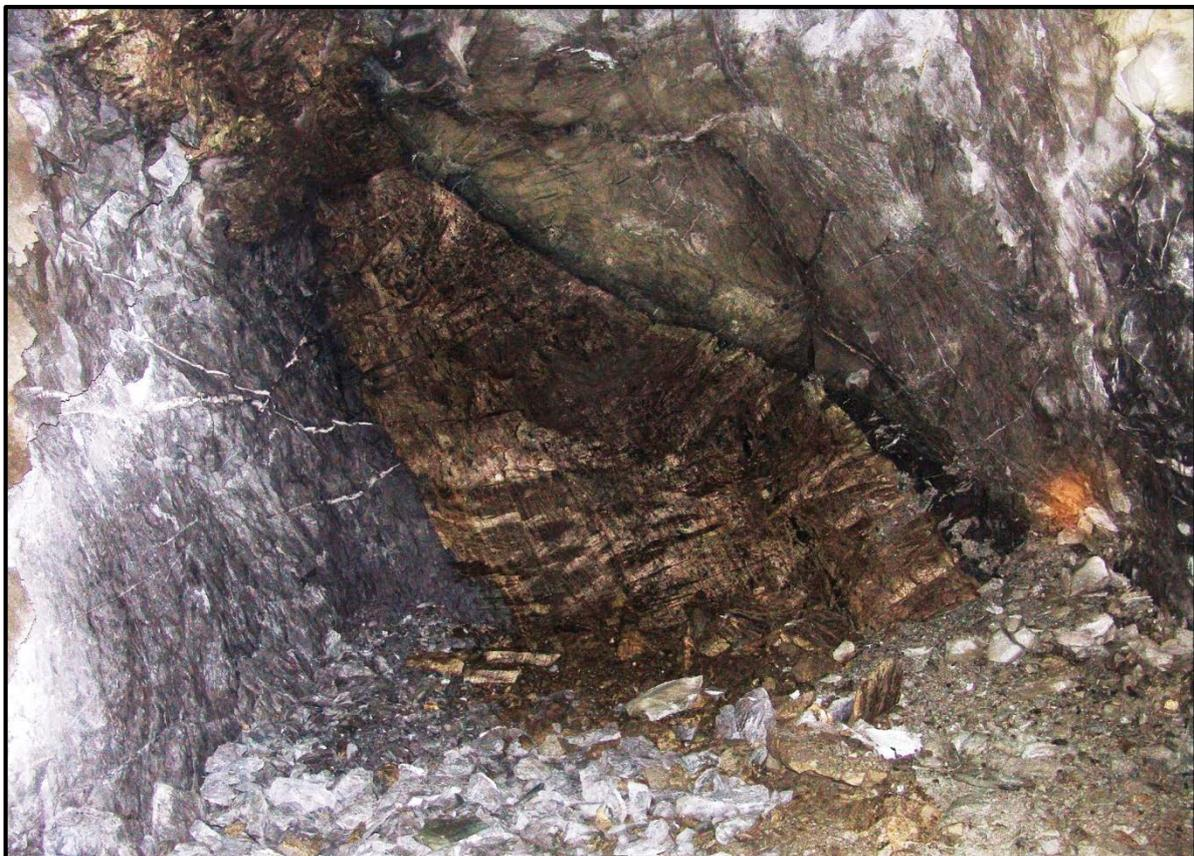
Figure 2: Goose 10170 level (now mined) showing high grade massive nickel sulphide (~13% Ni) in the ore drive.
