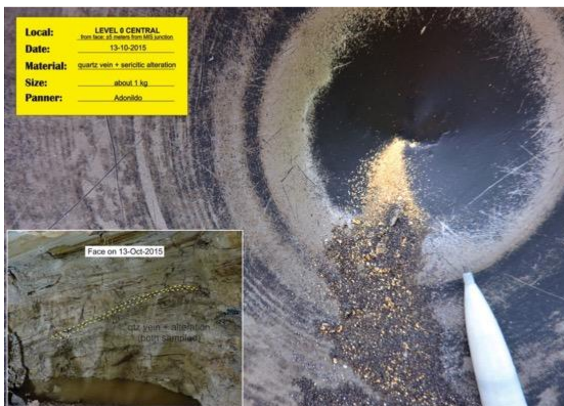
Figure 1. Panning of a 1kg sample consisting of vein and alteration from the face of Level 0 Central approximately 2m beyond the assays reported in this announcement. Assays from the corresponding panel samples taken from the walls are pending.
