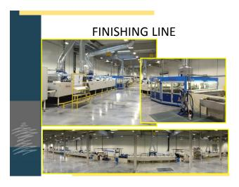
The leather finishing process applies the colour and chemical mix to the hide. Consistency of the application and minimisation of wastage are key objectives. In between applications, the hide is dried using infra-red technology.
