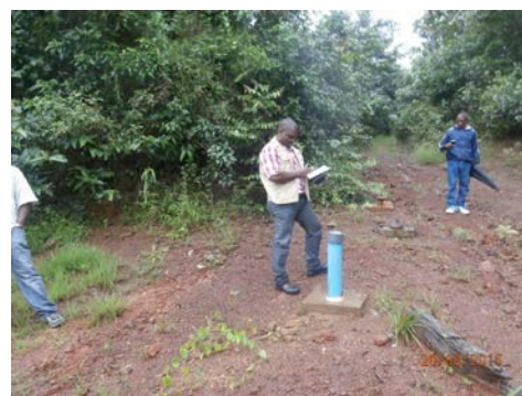
Fig 2 | Dipping a piezometer for ground water level monitoring
