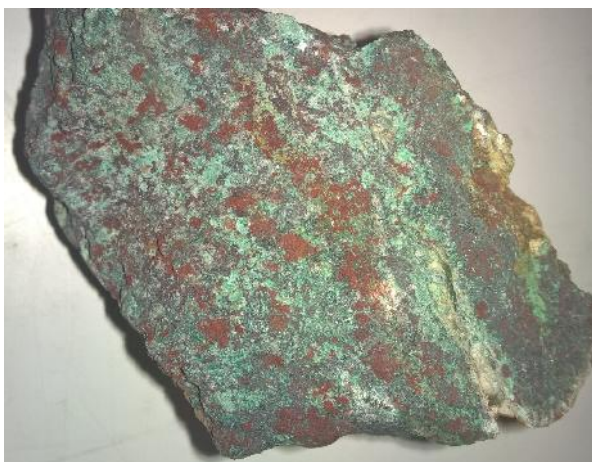
Figure 5. Bridget gossan (sample P702407) showing abundant malachite and iron oxides after sulphides; 19.25% Cu, 0.38 g/t Au and 10.8 g/t Ag.
