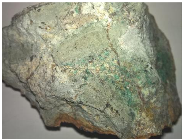
Figure 6. Altered basalt, Bridget prospect (sample P702405) with hairline quartz stockworking, intense silica-sericite-epidote alteration and malachite after remnant sulphides; 0.75% Cu and 0.13 g/t Au.
