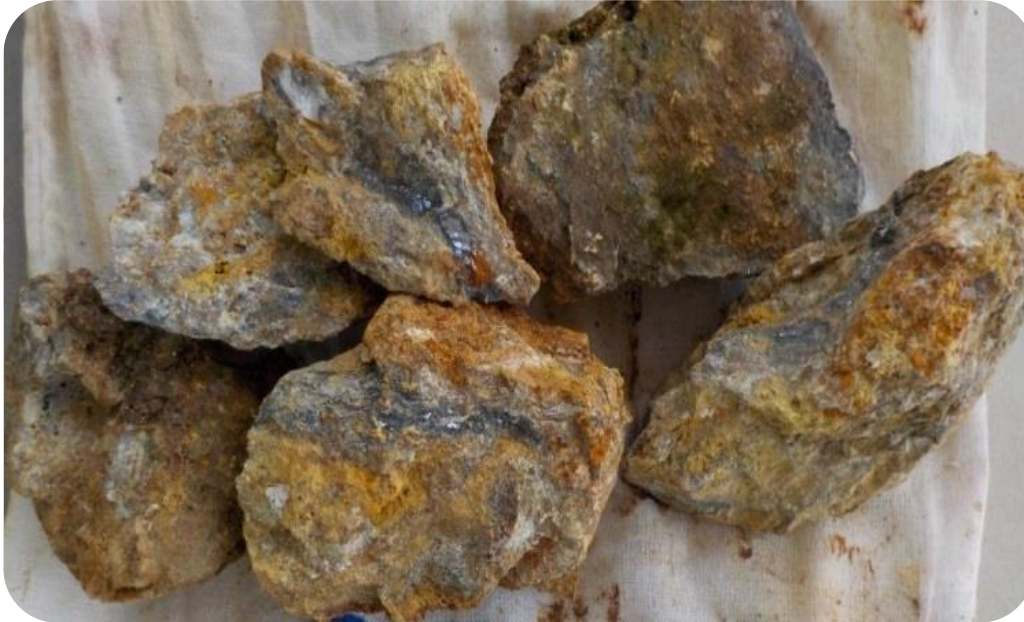
Image One: SKTL003 gossanous vein from Thali North breccia zone comprising mainly secondary lead minerals with relict galena bands, assay 0.2% Cu, 27% Pb and 1,860g/t Ag.
