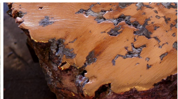
Above right: sulphide copper ore (chalcopyrite) commences just 12m from surface; and unique large (130kg) native copper mass cut to reveal near solid copper metal core. A pervasive native copper rich supergene zone continues from near surface to depths of up to 180m in some places.
