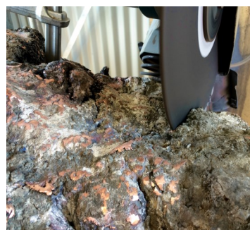
Above right: sulphide copper ore (chalcopyrite) commences just 12m from surface; and unique large (130kg) native copper mass cut to reveal near solid copper metal core. A pervasive native copper rich supergene zone continues from near surface to depths of up to 180m in some places.
