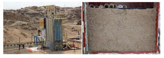
Integrity of the agglomerates (as shown on the right above) was again clearly evident during the unloading process and no percolation issues were observed.
