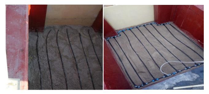
Leach irrigation was conducted for 20 days followed by a post leach drain of 2 days and then a rinse and post rinse drain phase of 3 days and 5 days respectively. A weak sulphuric acid solution (2g/l) was used as rinse solution.
