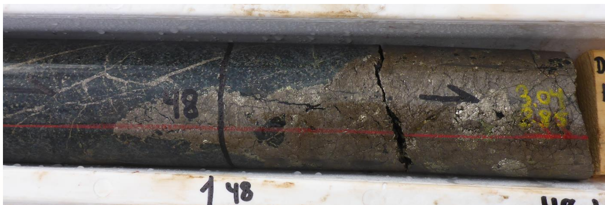
Figure 5 – Close up core photo of irregular top contact of massive sulphide vein in DMDD0004 at Conductor D. Interval (0.5m downhole) assayed 8.14% Ni. Note core is HQ3, with a diameter of ~61.1mm.
