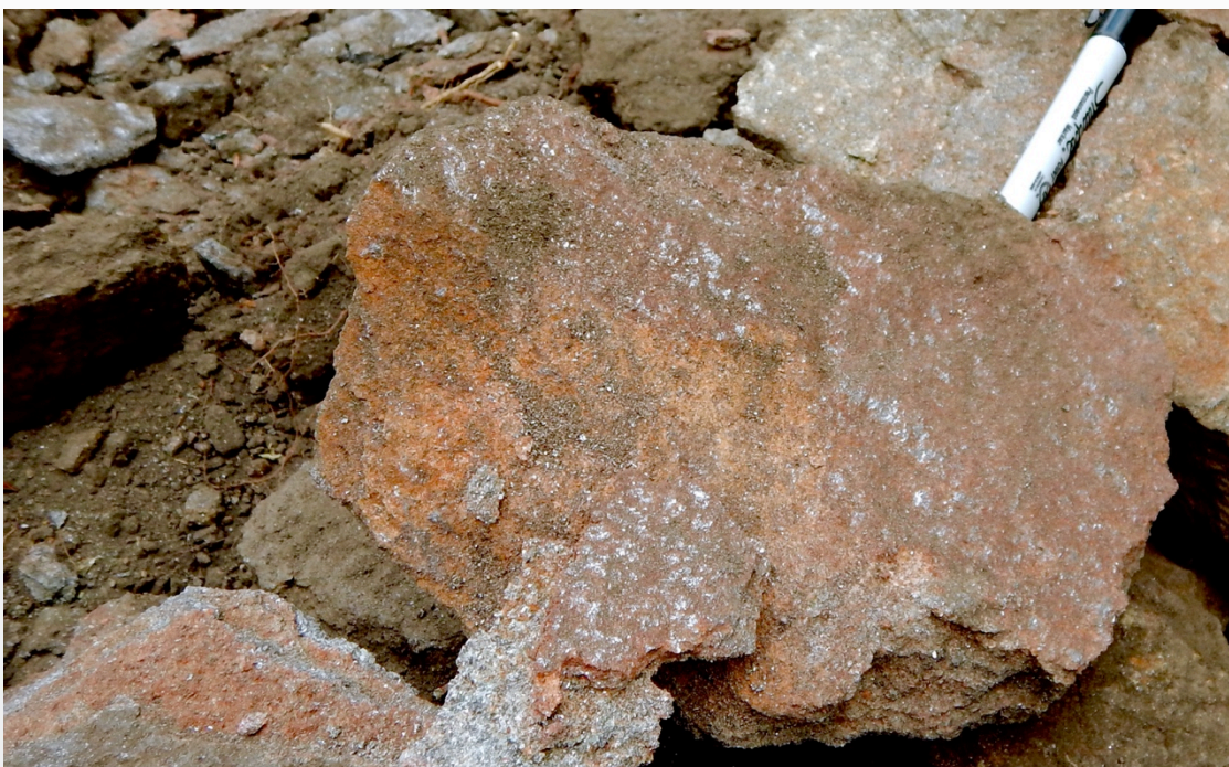
Photos 1,2. Top: Outcropping graphitic schist on Ulanzi north ridge adjacent to where the 29% TGC bulk sample was collected. Bottom: Photo of bulk sample being collected. Graphite is quite visible on surface of rocks.
