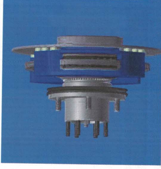
Outer Polymer Cover removed
