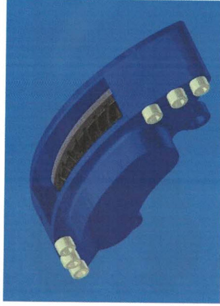
Aluminium cast calliper
