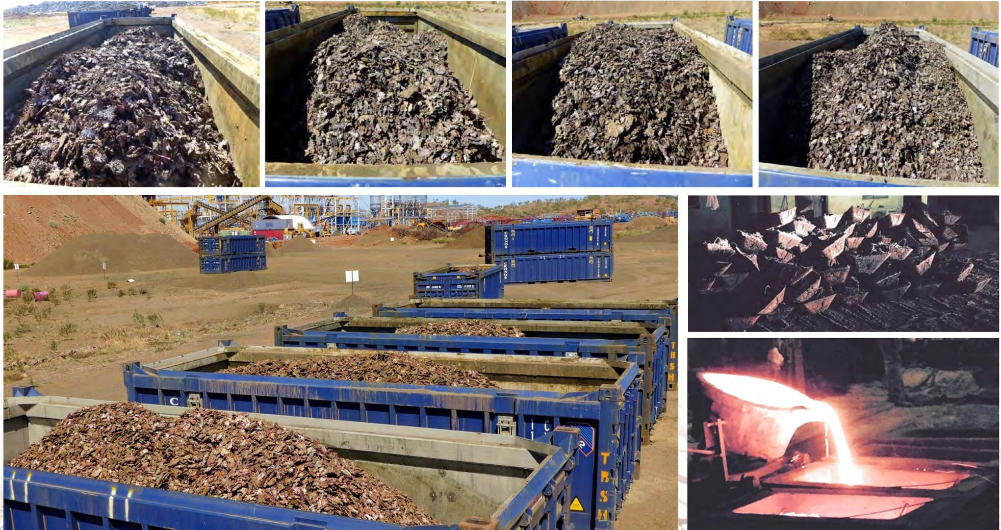
*Coarse native copper product ranging in grade from 85-95% copper metal in concentrate, produced from crushing and screening. The purpose of this circuit is to remove oversize native copper (+40mm) prior to commencement of processing in main mineral processing plant under construction. Trial processing of containers of native copper concentrate successfully produced a final product grade of 99.67% Cu.*
