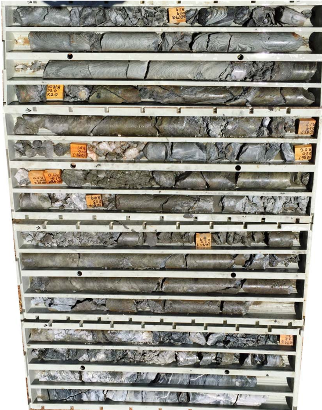
Figure 1: Photos of core from 79.4m in CODD001 illustrating copper mineralisation in massive, semi-massive and vein type mineralisation from 81.4m – 99.8m
