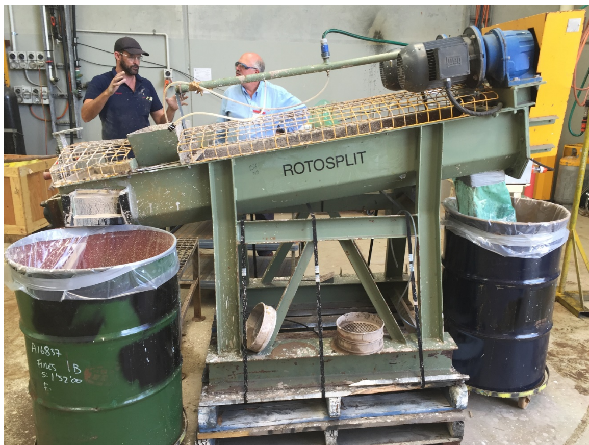
Figure 6: Continuous log washer trials on kaolin clay material from Mulga Rock
