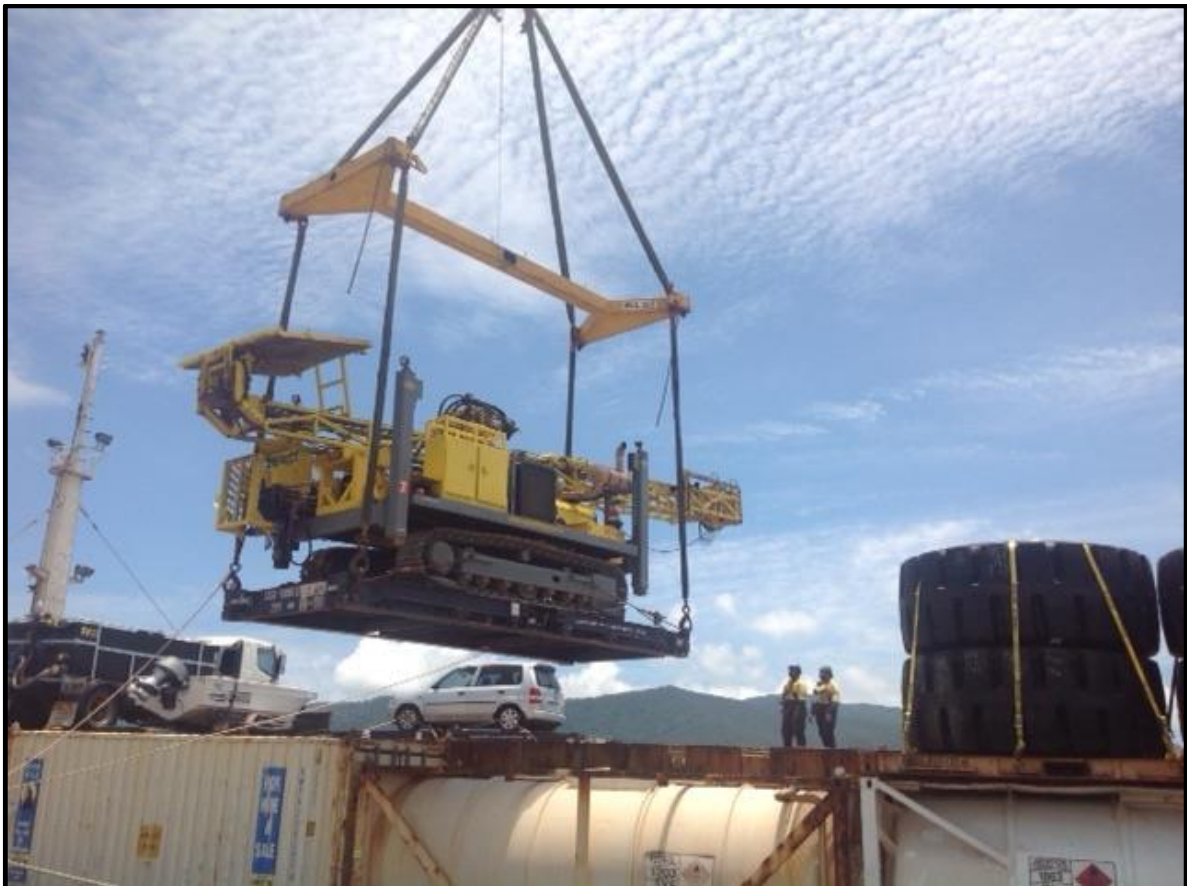
Eagle Drilling NQ track mounted diamond core drill rig being craned on to Seaswift vessel, Trinity Bay, in Cairns yesterday
