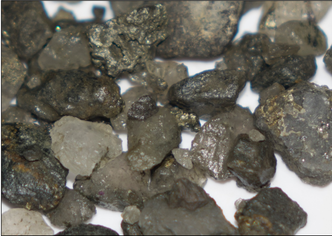
Figure 3: RC chips from YARC001 showing intense pyrite, quartz, sericite alteration and mineralisation.
