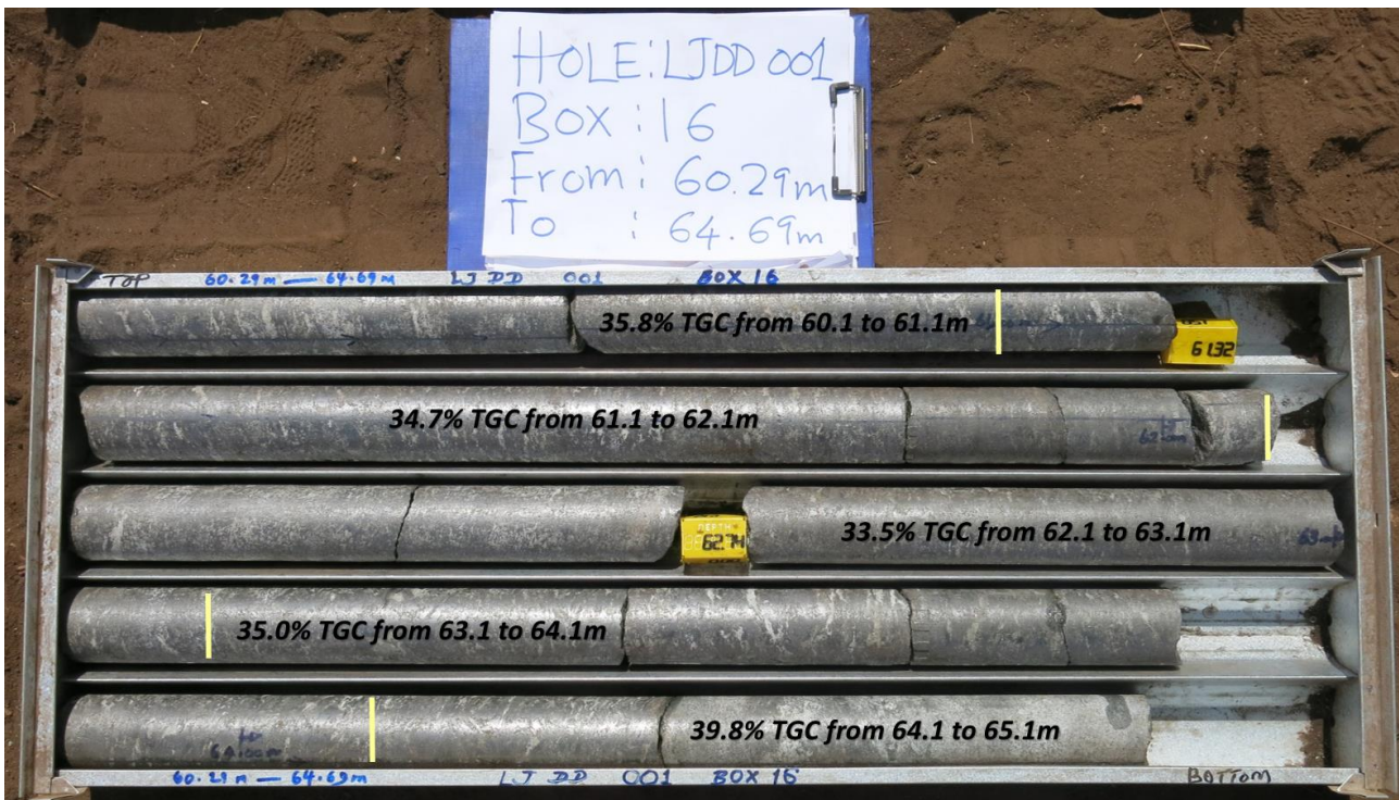
Image 1: Photo of diamond drill core showing spectacular grades within the graphite schists. The above core tray forms part of a wide, high grade intersection of 20m @ 20.5% TGC from 50.1m.
