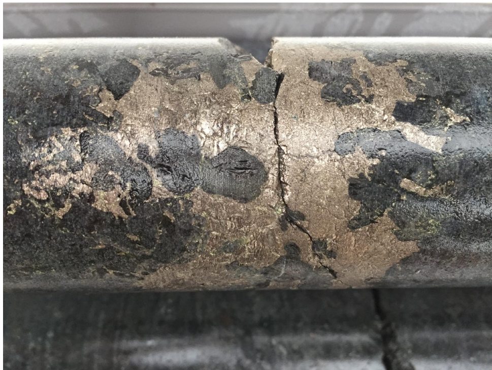
FIGURE 2: Core from MRDD010 showing stringer sulphides at depth 179 metres. Note the sulphides encasing large olivine and pyroxene crystals. Portable handheld Niton XRF readings range from 1.5% up to 5.4% nickel and from 0.2% up to 1.2% copper.
