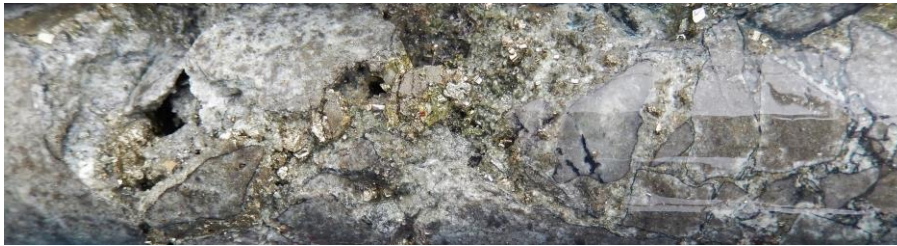
Figure 3i: LEFT Core photo at 607.6m showing tourmaline breccia. The clasts are very highly altered and the matrix is rich with pyrite, arsenopyrite and chalcopyrite.
