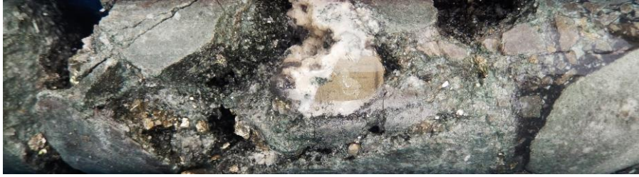
Figure 3g: LEFT Core photo at 575.8m showing tourmaline breccia with drussy quartz-carbonate complexes (dQtz-Carb) and sulphides as matrix material. Sulphides include pyrite, arsenopyrite and chalcopyrite.
