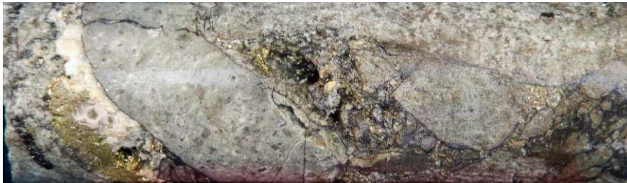
Figure 3j: LEFT Core photo at 613.0m showing tourmaline breccia. The clasts are more tightly packed and the sulphides are increasing pyrite and chalcopyrite. This indicates a "root" position of the breccia.
