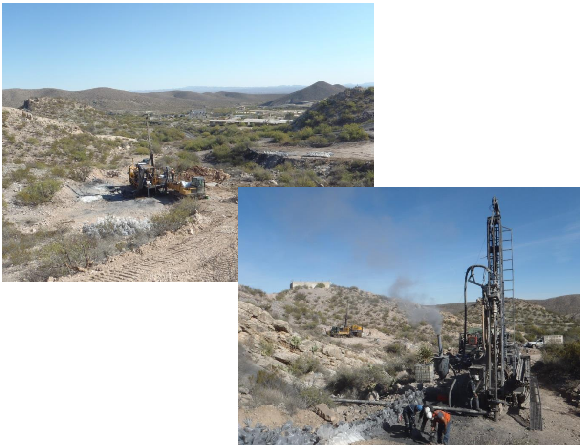
Figure 3. Tres Amigos surface drilling (diamond and RC rigs) showing old ASARCO township in the background.
