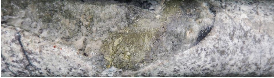
Figure 2a: LEFT core photo at 759.6m showing brecciated porphyry with pyrite/chalcopyrite matrix with drussy quartz (drussy quartz means quartz that occurs in cavities and is typically crystalline).
