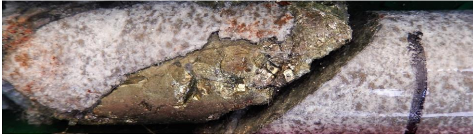
Figure 2b: LEFT core photo at 792.95m showing chalcopyrite vein cutting through porphyry, which contains disseminated chalcopyrite and pyrite.
