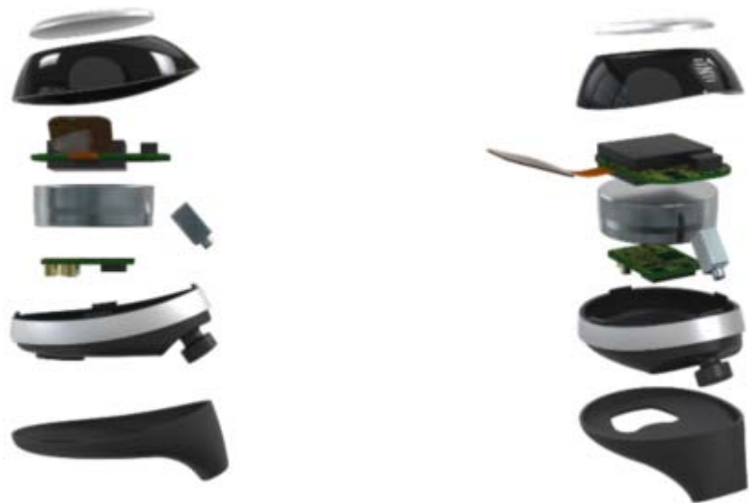
Figure 1 - Diagrammatic representation of preliminary ear-bud hardware design
