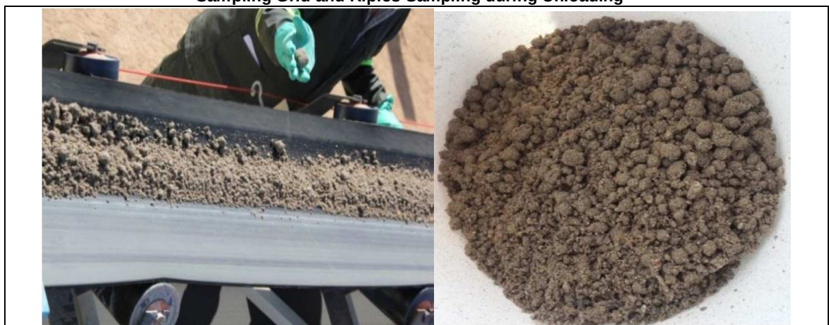
Figure 13.30 Sampling Grid and Ripios Sampling during Unloading
